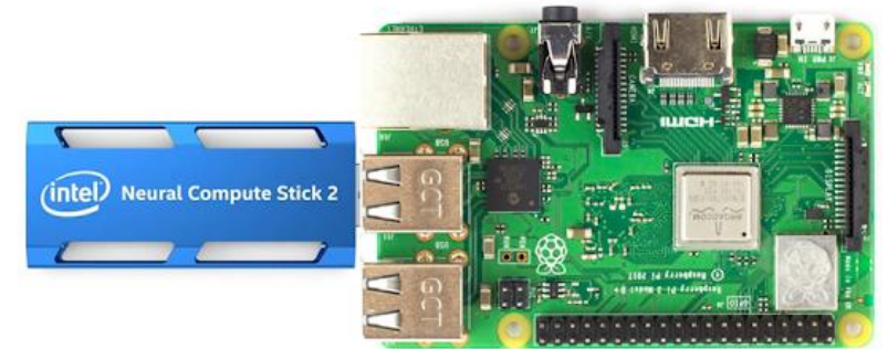
Raspberry Pi 3B + Intel Neural Compute Stick 2
